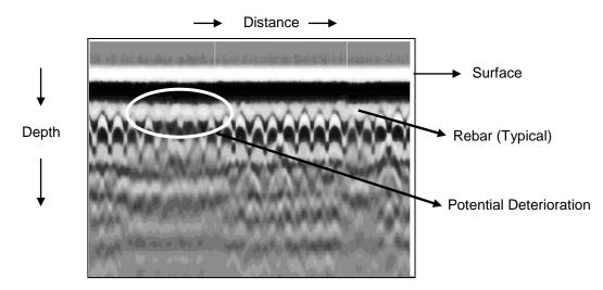
Figure 5.10.1-1: Typical Radar Output Image with Notations.
