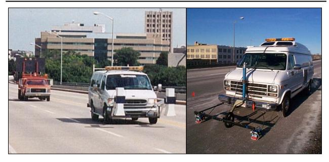
Figure 5.10.1-2: Horn Style (left) and Contact Style (right) Vehicle-Mounted Transducers.
