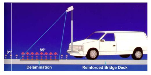
Figure 5.11.1-2: Illustration of IR of a Bridge Deck.
