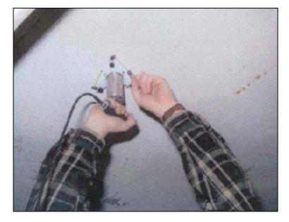
Figure 5.12.1-2: Inspector Using an Impact Echo Test Unit.
