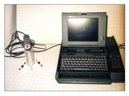
Figure 5.12.1-1: Impact Echo Test Unit.
