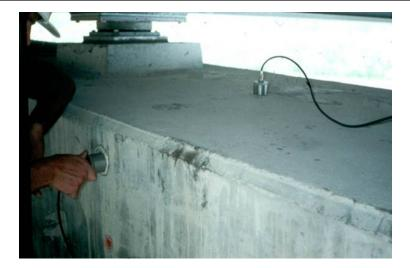
**Figure 5.13.2-1:** Inspector Conducting UPV on a Concrete Pier Cap Using Semi-Direct Transmission.
