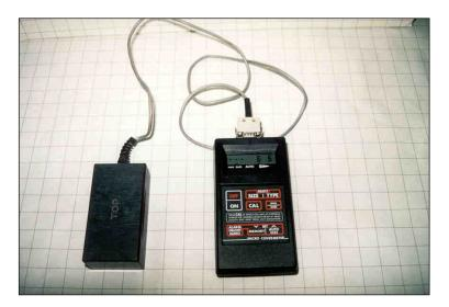
Figure 5.14.1-1: View of a Basic Covermeter Unit.
