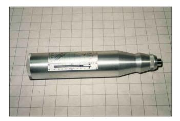
Figure 5.18.1-1: Standard Rebound Hammer.
