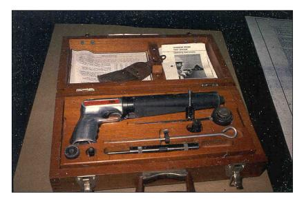
Figure 5.19.1-1: Windsor Probe Test Kit.
