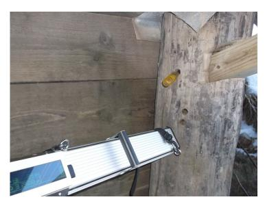
Figure 5.20.2-1: IML Resistograph, note the other old borings from a regular drill
