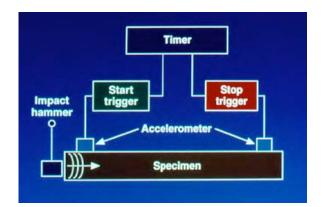
Figure 5.21.2-1: Schematic of a Stress Waver Timer
