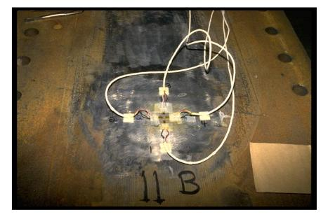
Figure 5.22.1-2: Strain Gauges Attached to the Steel Track Casting of a Movable Bridge.
