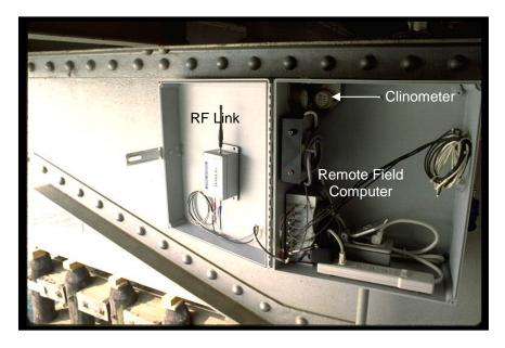
Figure 5.22.1-1: Remote Field Computer, Clinometers, and RF Link Mounted in Protective Enclosure.
