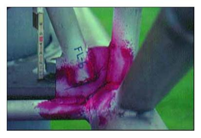
Figure 5.4.1-2: Gusset Plate with Applied Dye Penetrant.
