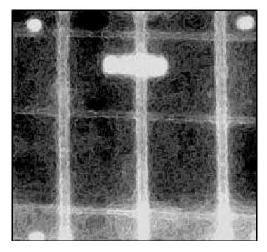
Figure 5.9.1-3: RT image of concrete slab. Note reinforcing layout shown on film.
