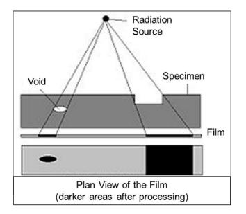
Figure 5.9.1-1: RT of material with a void and notch. Note the darker areas on the film located below the test material.
