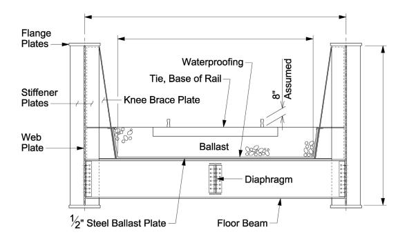
Figure 38.3-2 Typical Section of Through-Girder Bridge (Two-Way Floor System) WisDOT Bridge Manual
