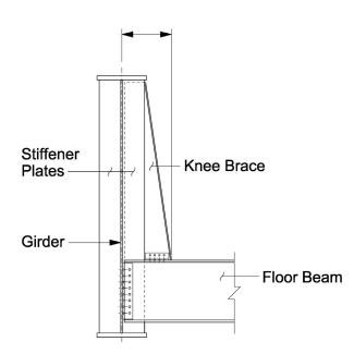
Figure 38.3-3 Knee Brace for Through-Girder Bridge
