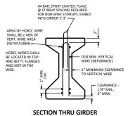
SHOWING WELDED WIRE FABRIC (WWF) STIRRUPS ASTM A1064 (FY = 70 KSI)
