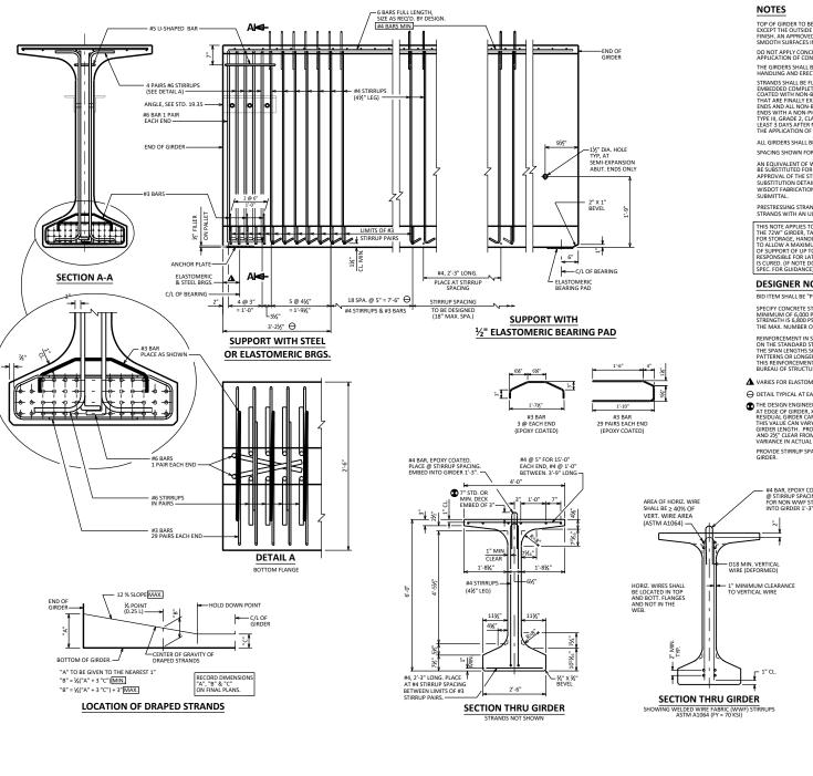
TOP OF GIRDER TO BE ROUGH FLOATED AND BROOMED TRANSVERSELY, EXCEPT THE OUTSIDE 15" OF GIRDER, WHICH SHALL RECEIVE A SMOOTH FINISH. AN APPROVED CONCRETE SEALER SHALL BE APPLIED TO ALL SMOOTH SURFACES INCLUDING THE OUTSIDE 15" OF THE TOP FLANGE. DO NOT APPLY CONCRETE SEALER OR EPOXY TO SURFACES RECEIVING APPLICATION OF CONCRETE STAINING.
