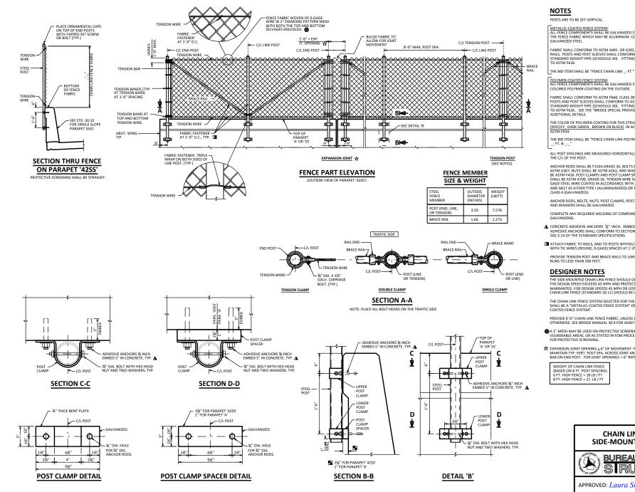
METALLIC-COATED FENCE SYSTEM: ALL FENCE COMPONENTS SHALL BE GALVANIZED STEEL, EXCEPT THE FENCE FABBIC WHICH MAY BE ALUMINUM- COATED STEEL OR
