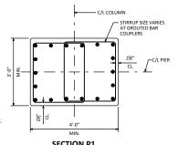
SECTION P1 (PRECAST PIER COLUMN REINF. TO BE DESIGNED BY DESIGN ENGINEER)
