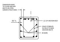
SECTION P2 (PRECAST PIER CAP REINF. TO BE DESIGNED BY DESIGN ENGINEER)
