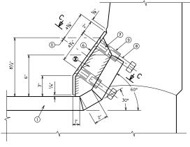
SECTION A-A SLOPED FACE PARAPET
