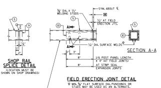
PROVIDE ¾" DIA. DRAIN HOLES IN LOW END OF ALL RAILS, CLEAR OF SPLICE SLEEVE.
