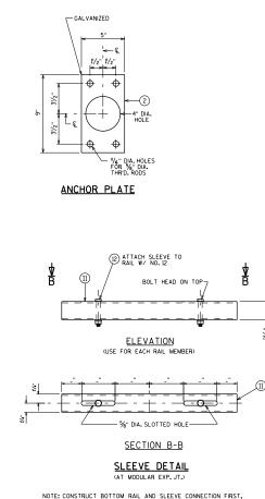
NOTE: CONSTRUCT BOTTOM RAIL AND SLEEVE CONNECTION FIRST, THEN MIDDLE RAIL, AND THEN TOP RAIL, TO ALLOW EASE IN PLACEMENT OF BOLT NO. 12.
