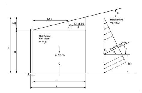
Figure 14.4-3 MSE Walls Earth Pressure for Sloping Backfill (Source AASHTO LRFD)
