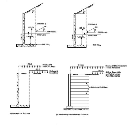
Figure 14.4-8 Application of Load Factors (Source AASHTO LRFD)
