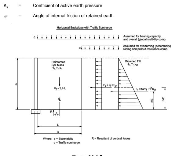
Figure 14.4-2 MSE Walls Earth Pressure for Horizontal Backslope with Traffic Surcharge (Source AASHTO LRFD)
