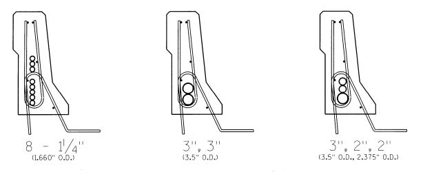
Figure 30.4-1 Maximum Allowable Conduits in "\_\_SS", "HF" and "LF" Parapets
