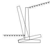
LIMITING ECCENTRICITY (FAILURE DUE TO OVERTURNING)
