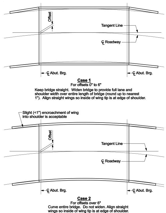
Figure 3.2-1 Bridge Layout on Horizontal Curves
