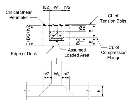
Figure 17.6-6 Assumed Load Distribution for Punching Shear
