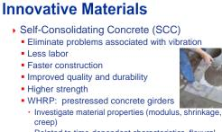
Related to time-dependent characteristics, flexural stiffness change, prestress losses
