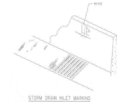
Figure 1. Typical Installation of Storm Drain Inlet Marking
