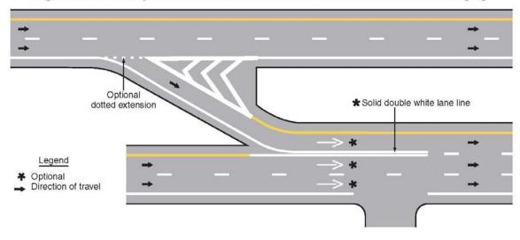
Figure 3B-12. Example of Solid Double White Lines Used to Prohibit Lane Changing
