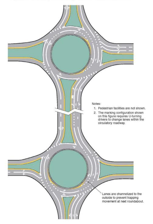
Figure 3C-13. Example of Markings for Two Linked Roundabouts
