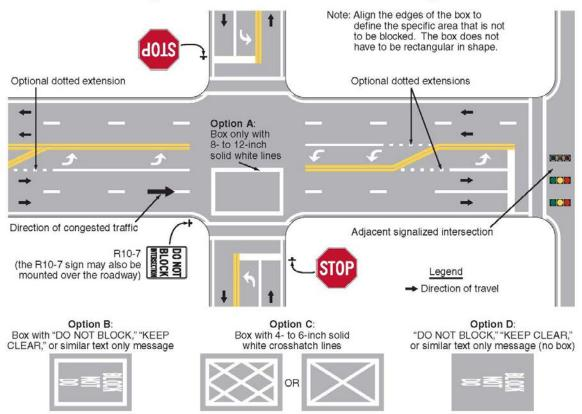
Figure 3B-18. Do Not Block Intersection Markings
