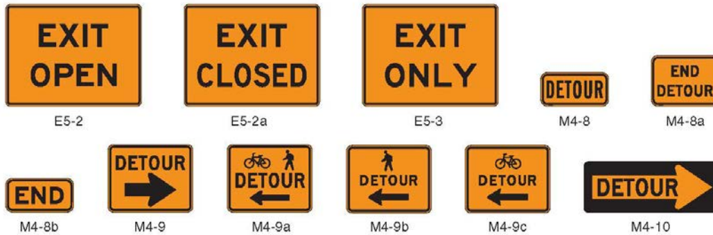
Figure 6F-5. Exit Open and Closed and Detour Signs
