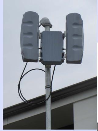
Bluetooth detection Providing real time travel times or freeways and arterials
