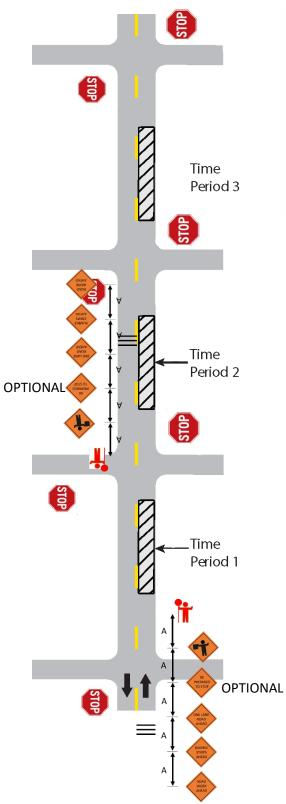
Sign spacing and temporary portable rumble strip placement Speed limit Spacing "A" 20–30 mph 200' 35–40 mph 350' 45–55 mph 500'
