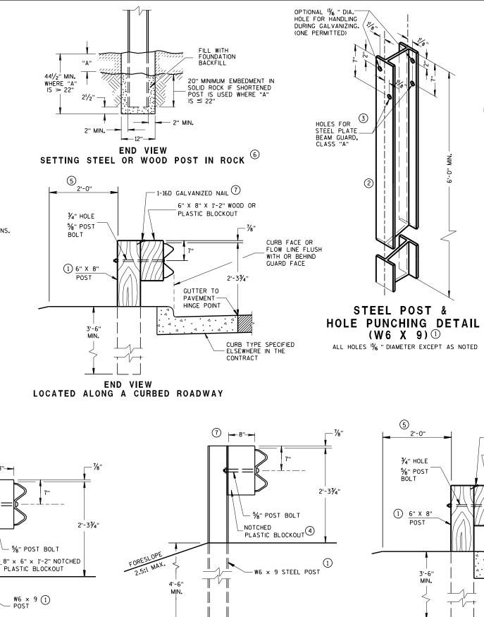
END VIEW STEEL POST & NOTCHED PLASTIC BLOCKOUT ALTERNATIVE STANDARD INSTALLATION
