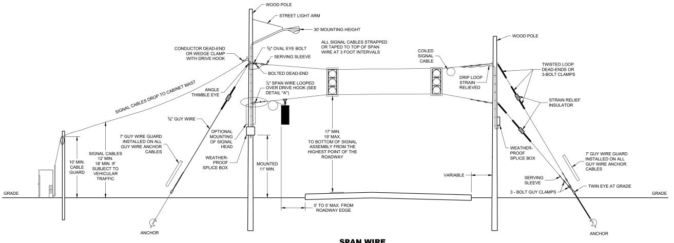
SPAN WIRE TEMPORARY SIGNALS
