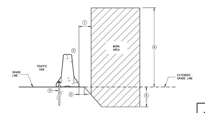
ANCHORED BARRIER SPACE REQUIREMENTS ON SLOPES
