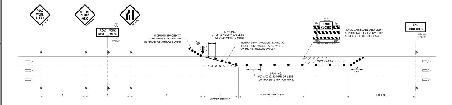
POSTED SPEED LIMIT ADVANCE TAPER LENGTH | BUFFER PRIOR TO WORK WARNING SIGN (12 FT. LANE) SPACE STARTING (MPH) SPACING (A) FEET (L) FEET (B) FEET 25 200' 125' 55' 30 200' 180' 85' 35 350' 245' 120' 40 170' 350 320' 45 500' 540' 220'
