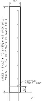
NOTE: USE GRADE C CONCRETE AT NE AND SE MASK WALLS.
