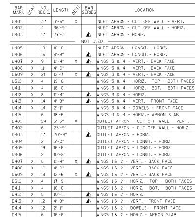
⚠ LENGTH SHOWN FOR BAR IS AN AVERAGE LENGTH AND SHOULD ONLY BE USED FOR BAR WEIGHT CALCULATIONS. SEE BAR SERIES TABLE FOR ACTUAL LENGTHS.
