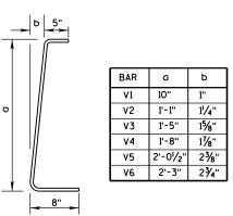
4V BARS 2 AT EACH SIZE REQUIRED FOR STIRRUP ASSEMBLY
