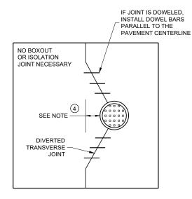
MANHOLE WITH DIVERTED TRANSVERSE CONTRACTION JOINT
