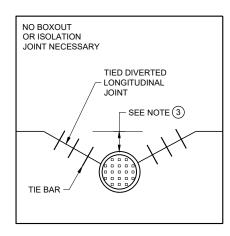
MANHOLE WITH DIVERTED LONGITUDINAL CONTRACTION JOINT
