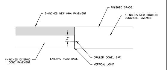
ASPHALT TO CONCRETE PAVEMENT TRANSITION
