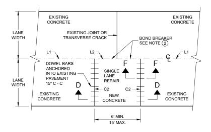
**PLAN VIEW SINGLE LANE CONCRETE PAVEMENT REPAIR**
