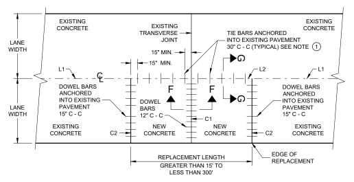
**PLAN VIEW** SINGLE LANE CONCRETE PAVEMENT REPLACEMENT
