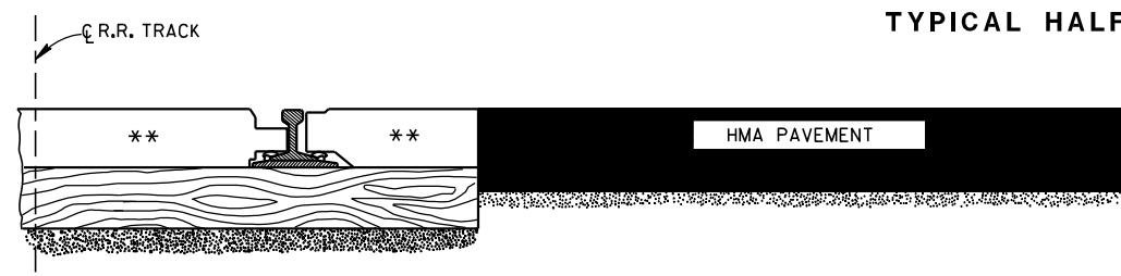
SECTION A-A HMA PAVEMENT APPROACH
